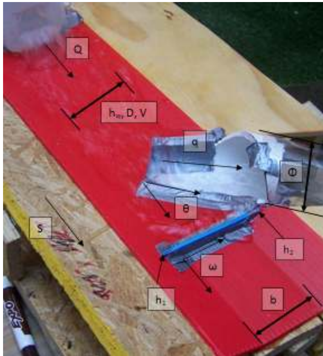
Figure 7: Bench top set-up with variables.
