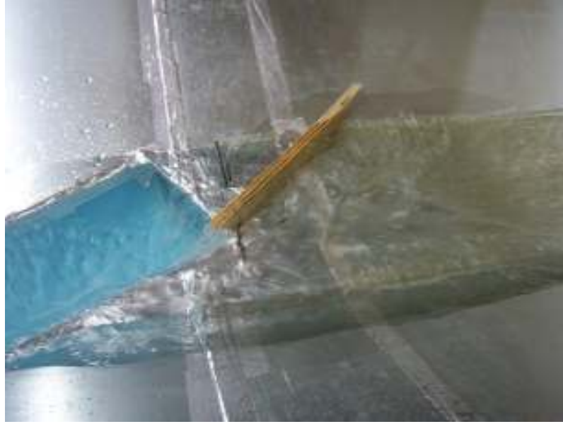
Figure 22: 30 degree pipe with 35 degree tapered vane.
