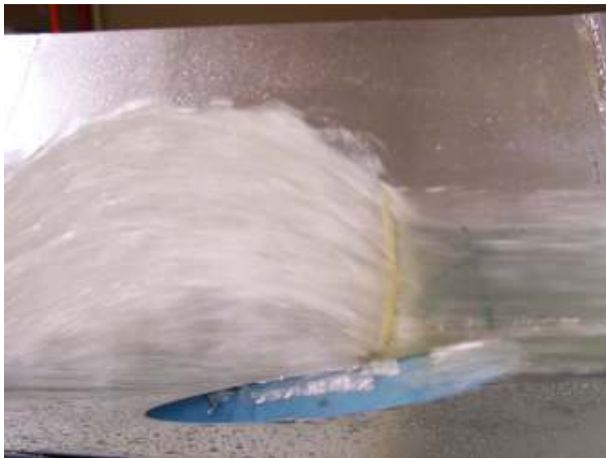
Figure 11: "Rooster tail" wave from vane
