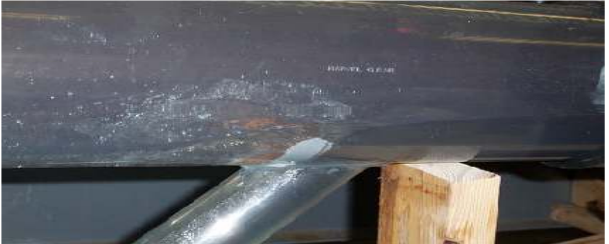
Figure 1: Smaller pipe on the bottom system with hydraulic jump (Coonrod, 2002).
