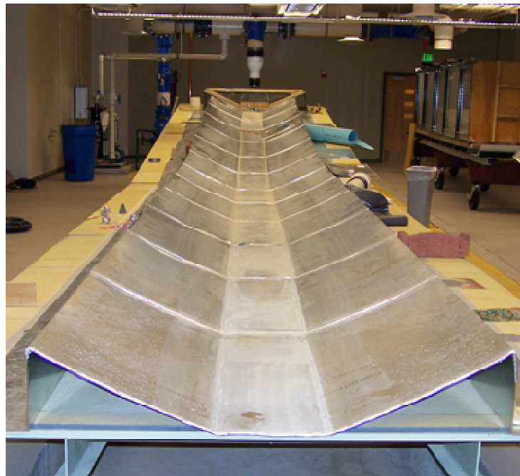
Figure 5: Side wall set-up on tilting table.
